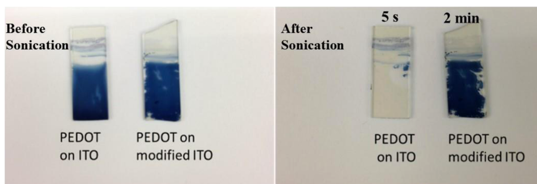
Figure 6. Optical images of PEDOT films on ITO and modified ITO before and after ultrasonication adhesion test. PEDOT on ITO was tested for 5 s and PEDOT on modified ITO was tested for 2 min.
